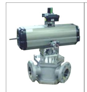
Dedicated lines for multiple products can be minimized using 3-way piggable valves. PBM's 3-way piggable cavity free valves can reduce the number of launchers and receivers required in a piping system. The smooth 120-degree turn through the PBM 3-way piggable valves permits easy diverting of a line pig used to clean the pipe or tubing lines.
