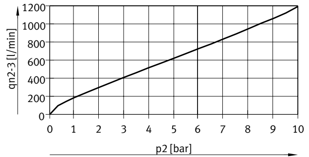
Flow rate q_n from 2 > 3 as a function of output pressure p_2
